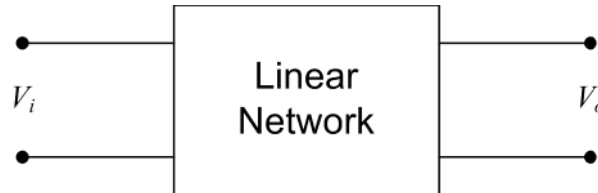
Figure 5.1: A two port linear network showing the input and output voltage signals.
